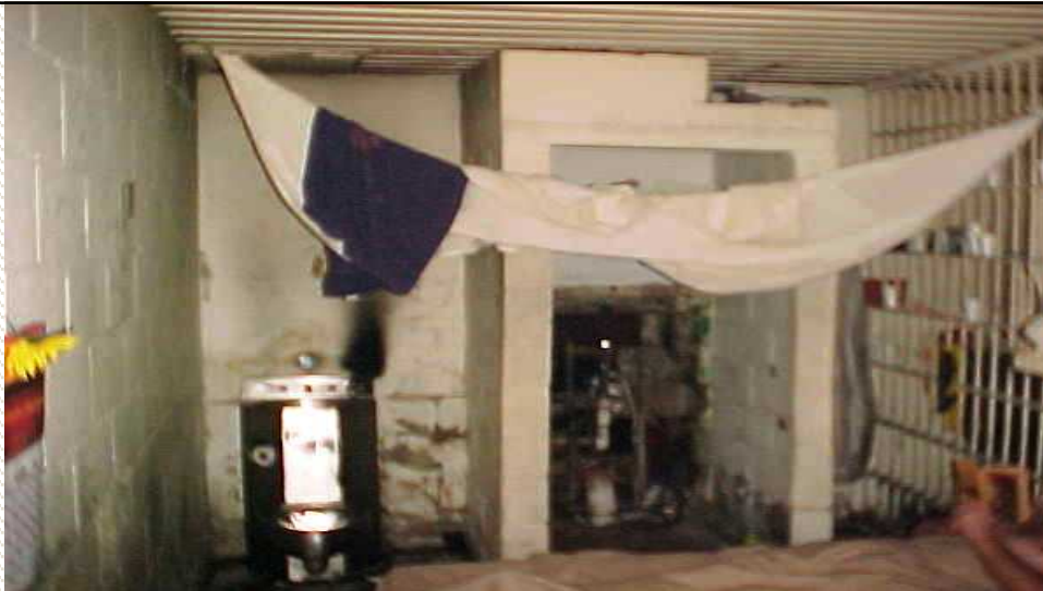
Flammable materials hanging from ceiling in men's cell block
